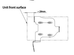
We recommend a distance about ~29 mm to the front surface of the double DIN head unit.
