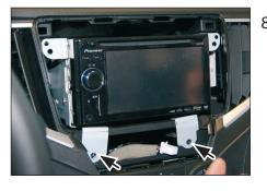
Connect all required circuit points and cables. Place head unit and fix it with with the OEM screws (see arrows)
