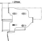
We recommend a distance about ~27mm to the pocket front surface of the 1-DIN head unit.
