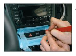
Use masking tape in order to protect the surface from scratches. (see photo)
